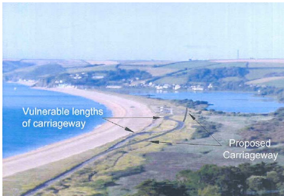
Figure 3-5 Diagram showing location of proposed A379 realignments
